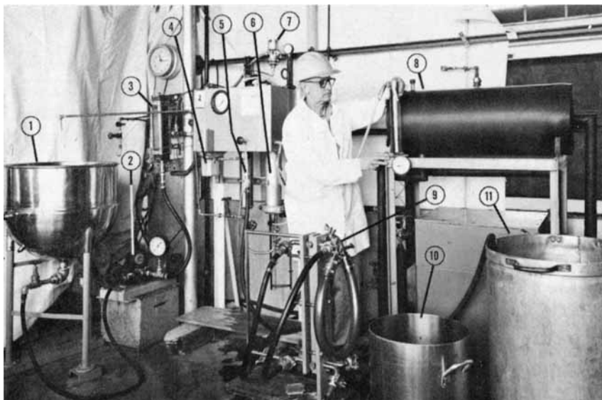
Fig. 1. Pilot plant reverse osmosis equipment: (1) feed tank, (2) booster pump, (3) flowmeter, (4) prefilter, (5) staged centrifugal pump, (6) pressure vessel, (7) low-pressure safety switch, (8) brine chiller, (9) plate heat exchanger, (10) concentrate collector, (11) permeate collector.
